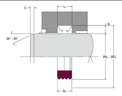
Technical DetailsMetricInchOperating conditionsMaximum speed0.1 m/sec0.3 ft/secTemperature range-30°C + 80°C-22°F + 76°FMaximum pressure350 Bar5000 p.s.i
